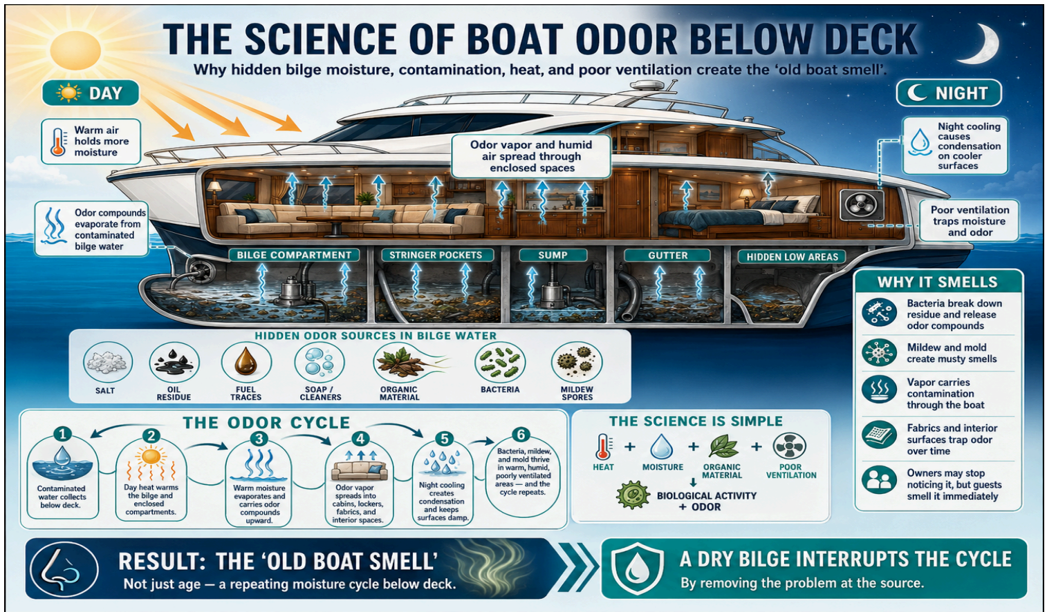
Figure 2.2 — The science of boat odor below deck.
